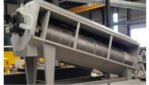
**With its longstanding industrial experience, Nijhuis Industries has developed a cost-effective screw press system (NSP) for sludge dewatering to deal with a wide range types of sludge. That being said, NSP unit is suitable to handle both biological and physical-chemical types of sludge.**
